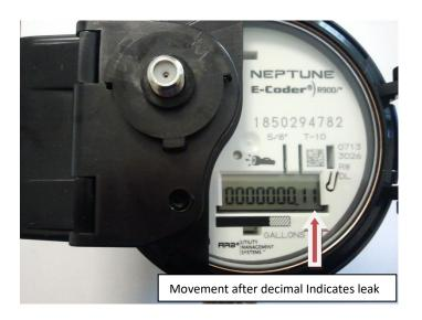
Neptune Meter- If you have a possible leak two things will occur 1.) An image of a faucet will appear on the display. 2.) The numbers after the decimal will be moving. Please allow 5 seconds for movement. If numbers do not appear, shine a bright flash light on the face of the meter and digits will appear.
