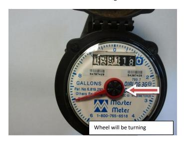
**Master Meter-** If you have a leak, the wheel in the middle of the meter will be turning.
